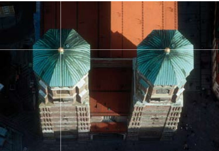
The origin of the Soldner coordinate system: the North Tower of the Frauenkirche in Munich
